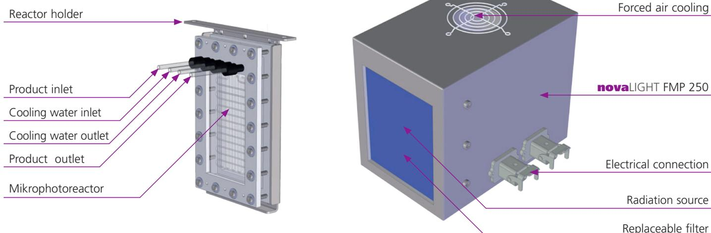
Due to the high pressure resistance, higher flow rates can be driven in the planar microphotoreactor than would be possible with a tube reactor.
