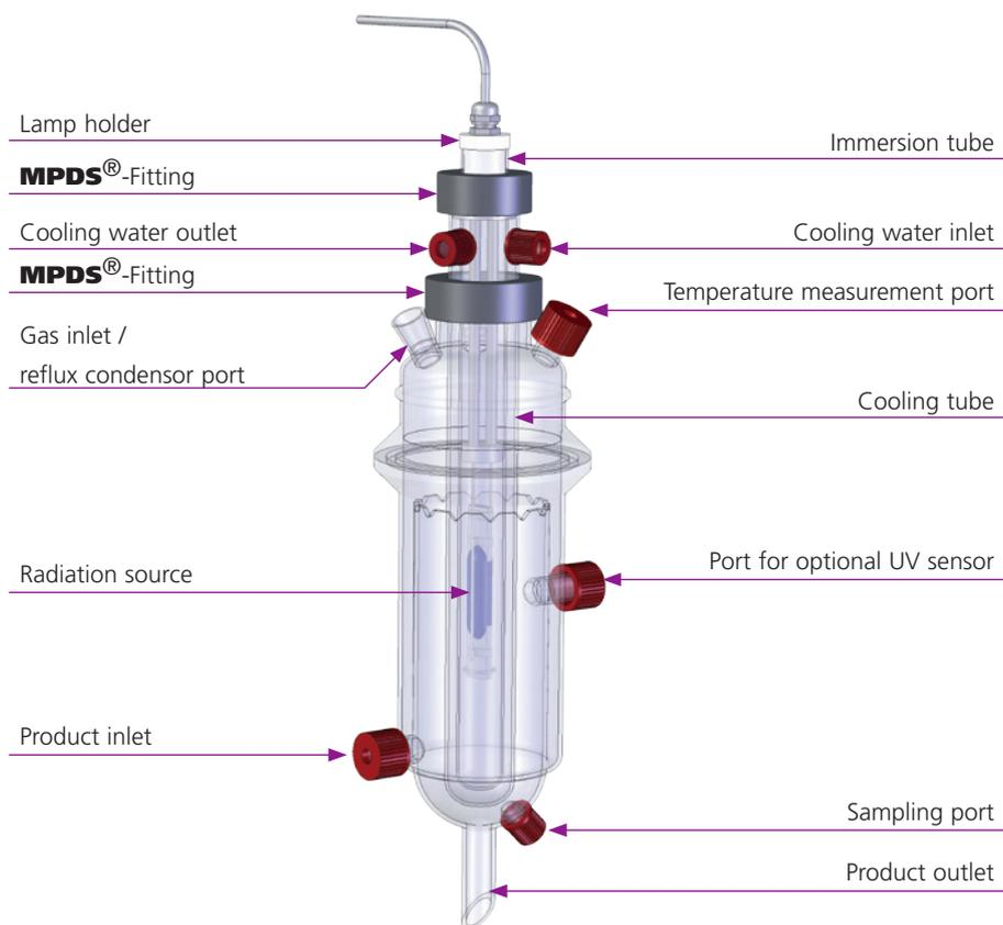
The falling film photoreactor from Peschl Ultraviolet GmbH has been optimised in such a way that the size of the irradiated surface (cm<sup>2</sup>) in relation to the intensity generated in the distance to the radiation source is ideal for most reactions. Since the immersion lamp system is not in direct contact with the reaction medium, photochemical and thermal polymerisations on the surface of the jacket tube are prevented.
